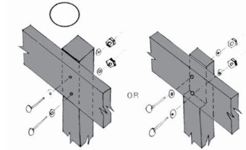
Fix joists to the bearers at max. 450mm spacing using triple grips or joist hangers, as shown in example below, and in accordance with manufacturers specifications.
