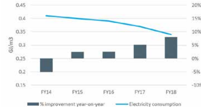
Figure 6: Electricity consumption and % Improvement per cubic metre of finished product
